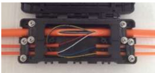
Routing A: direct way
